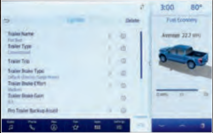
SIMPLE TRAILER SETUP Follow the Quick Start Guide to program one or more trailers into available Pro Trailer Backup Assist.
